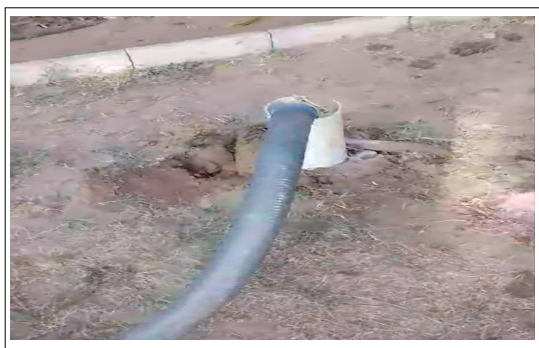
Fig 2: Shows how to take samples from wells using a water pump.
